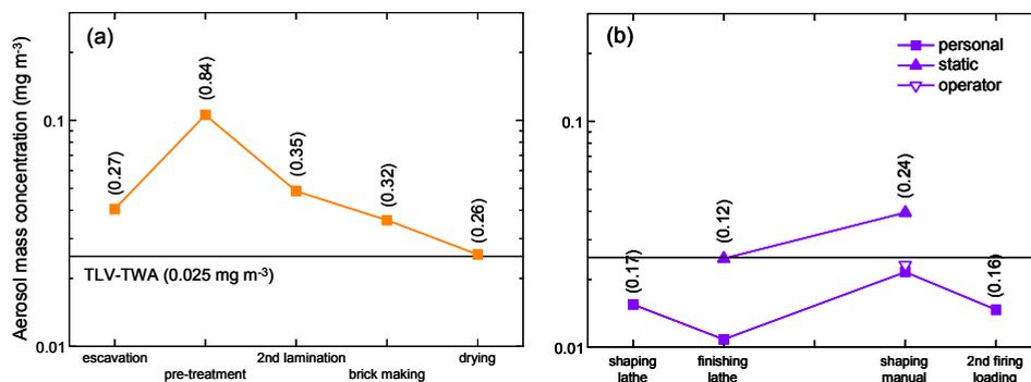
Fig. 2. Aerosol mass concentration of quartz in different working stations of clay brick (a) and pottery (b) productions. Data obtained from X-ray diffraction (INAIL, personal communication), after recalculation from the total respirable dust mass concentration (mean values, by gravimetry; data in parenthesis). In the plots the threshold limit value for the quartz aerosol mass concentration (TLV-TWA) is reported for comparison.
