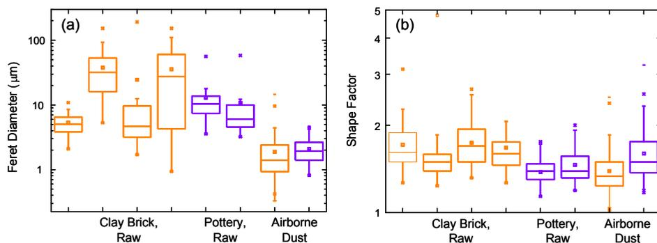
Fig. 1. Box and whisker diagrams of Feret diameter (a) and shape factor (b) of quartz grains from raw materials and airborne dust samples in clay brick (orange) and pottery (violet) productions.
