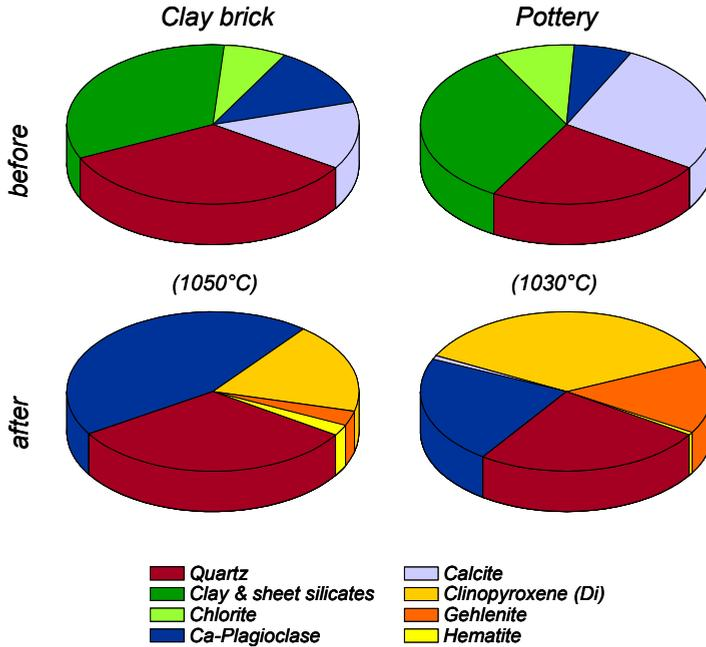
Fig. 3. Quantitative phase analyses of the crystalline species in clay brick and pottery raw materials before and after firing. The firing peak temperatures are reported in parenthesis.
