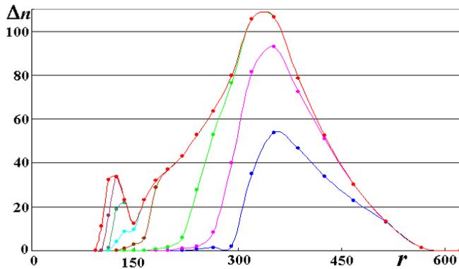
Fig. 7. Distributions of stripped droplets by sizes;  $r$  in  $\mu\text{m}$ . **Stony meteor.**  $V_\infty = 60$  km/sec,  $R_0 = 3.0$  mm,  $Re_\infty = 529$ ;  $GI = 43.5$ . Red – final distribution at  $\tau = 103$ ; blue, crimson, light-green, brown, light-blue, green, dark-brown – intermediate ones at  $\tau = 2.05$ ,  $\tau = 3.88$ ,  $\tau = 5.94$ ,  $\tau = 9.96$ ,  $\tau = 16.8$ ,  $\tau = 29.9$ ,  $\tau = 48.7$ ;  $\tau_{ch} = 1.45 \cdot 10^{-3}$  sec.
