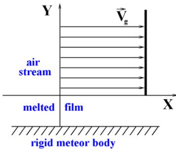
Fig. 1. Scheme of flow in ablation overtaking case.
