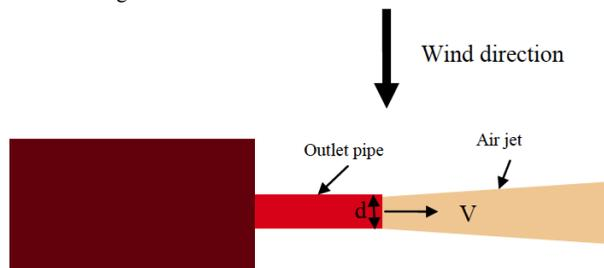
Fig. 2. Schematic of modelled source – plan view.
