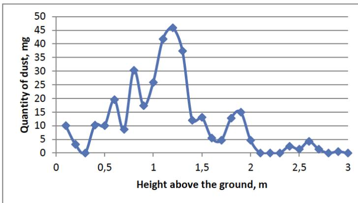
Fig. 8. Predicted airborne dust at 1 m downwind of the drill, based on the input variables in Table 2 and the distribution of terminal velocities measured in wind tunnel experiments.
