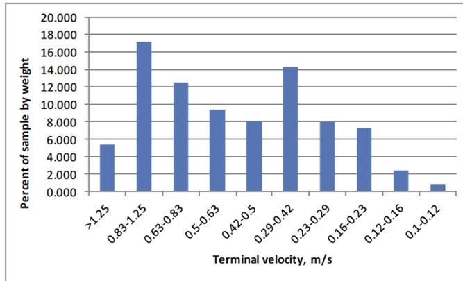
Fig. 5. Distribution of dust particles by terminal velocity.
