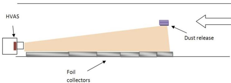
Fig. 3. Wind tunnel layout for measurement of terminal velocity or aerodynamic particle size distribution.
