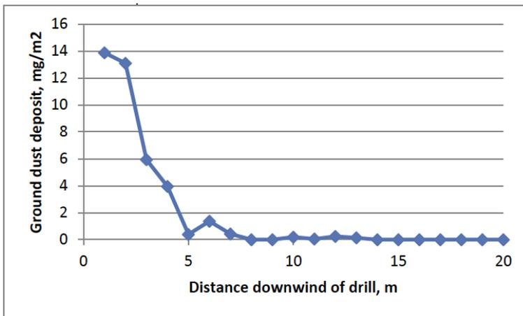
Fig. 7. Predicted ground deposit for example model run based on the input variables in Table 2 and the distribution of terminal velocities measured in wind tunnel experiments.
