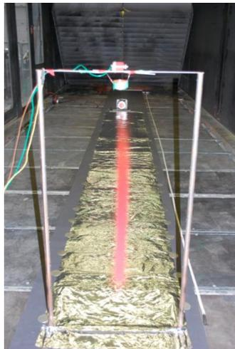
Fig. 4. Layout of experimental equipment showing the small sieve from which the dust is released at the top in the centre, the deposited stripe of pink dust down the centre of the foil collectors and the high volume air sampler at the end.
