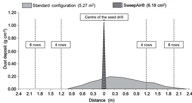
Fig. 5. Amount of dust in footprint area obtained with seed drill in standard configuration and equipped with SweepAir<sup>®</sup> kit.
