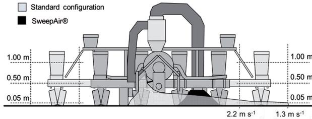
Fig. 4. Characteristics of the air stream generated by the fan of the Seeder in standard configuration and equipped with SweepAir<sup>®</sup> kit (front view of the machine).
