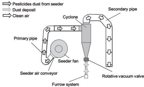
Fig. 1. Scheme of the main components of SweepAir® kit.
