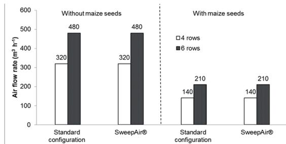
Fig. 2. Air flow rate measured with the machine in standard configuration and equipped with SweepAir® kit.
