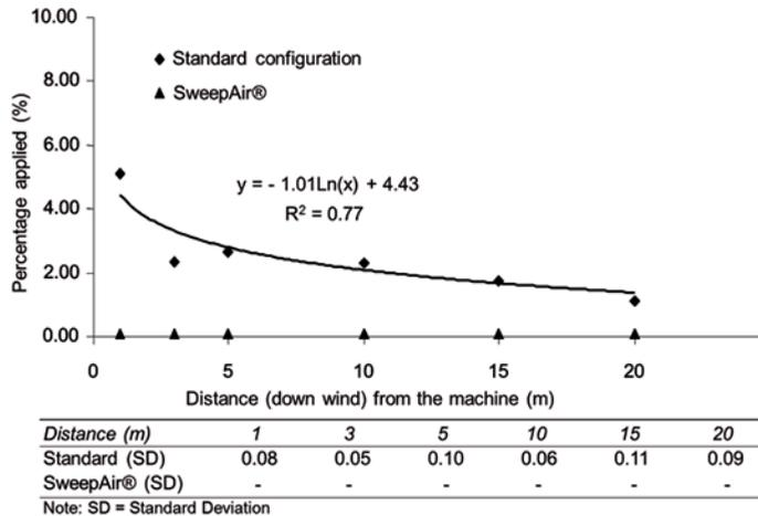
Fig. 6. Amount of drift material from the seeder in standard configuration and equipped with SweepAir® kit measured at different sampling distances.
