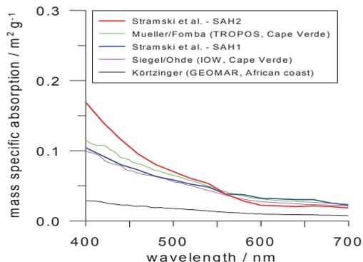
Fig. 6. Mass specific absorption coefficients of different dust samples.
