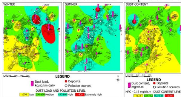
Fig. 2. Dust load levels and dust contents in Yerevan atmosphere.
