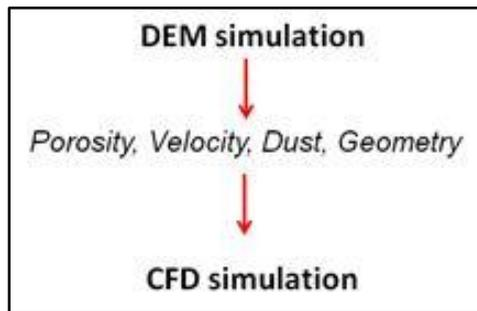
Fig. 1. Dust transport simulation process.
