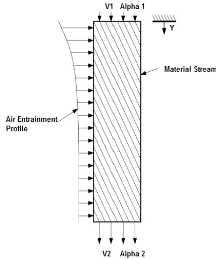
Fig. 2. Schematic diagram of air entrainment model.
