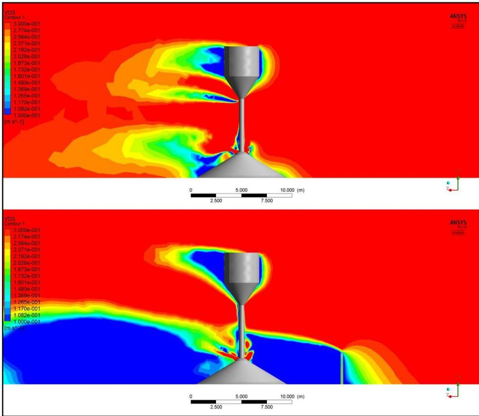
Fig. 3. Downstream velocity on centre plane. Top: stockpile no control. Bottom: stockpile with porous wind break.
