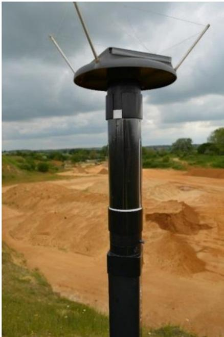
Fig. 1. A directional and depositional dust monitor.
