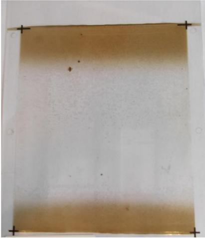
Fig. 1. A sealed directional sticky pad dust sample.
