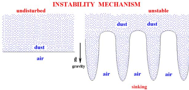
Fig. 3. The scheme of the aperiodic instability performance.
