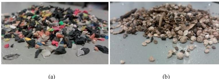
Fig. 2. Rigid plastic (a) and mixed wood/plastic scraps (b) used to replace conventional aggregates of mortars
