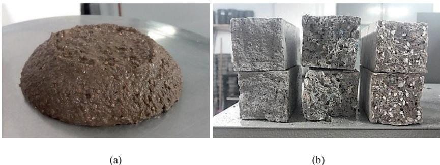
Fig. 3. Mortars based on AAB and CDW aggregates on fresh state (a) and after flexural tests (b)
