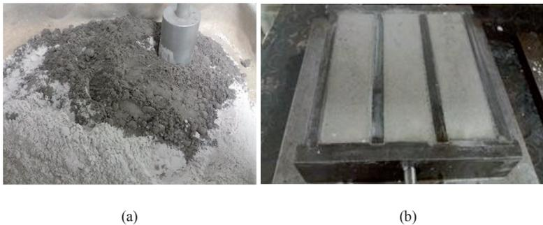
Fig. 1. PFA/GGBS mix used to replace conventional cement (a) and corresponding alkali activated binder used for mortars (b)
