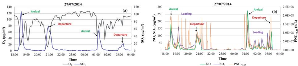
Fig. 2. Example of high resolution measurements with concentration peaks related to the different phases for (a)  $\text{O}_3$ ,  $\text{SO}_2$  and (b) NO,  $\text{NO}_2$  and  $\text{PNC}_{<0.25}$
