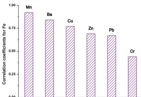
Fig. 4. Correlation coefficients of Fe concentration with traffic-related heavy metals Mn, Ba, Cu, Zn, Pb and Cr
