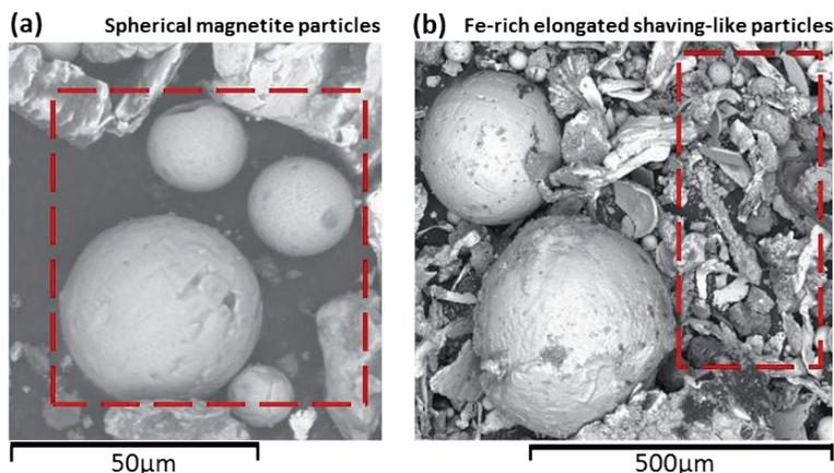
Fig. 3. Scanning electron microscopy observations (SEM) for indoor dust WB-41 selected from the samples of group 2 in Fig. 1.
