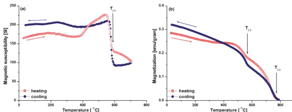
Fig. 2. Temperature dependence of magnetic susceptibility  $\kappa(T)$  curve (a) and induced magnetization  $M(T)$  curve (b).  $T_{C1}$  and  $T_{C2}$ , the Curie temperatures for magnetite and metallic iron, are marked, respectively
