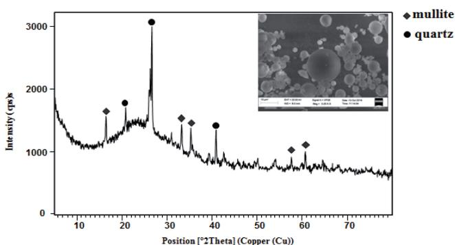
Fig. 1. XRD pattern and SEM image of fly ash
