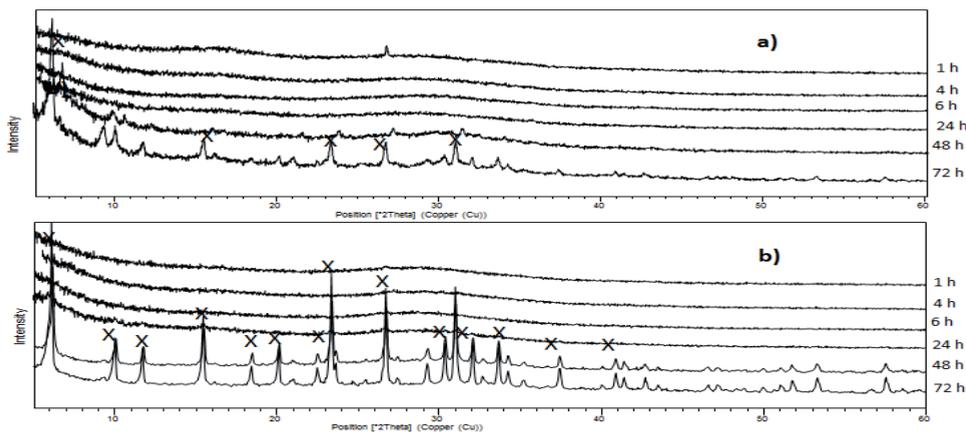
Fig. 2. X- ray diffraction patterns of synthesized zeolite at different time of crystallization, using distilled water, NaOH/FA 1.25, crystallization temperature 60 °C. a) without acid, b) with acid. X =X zeolite
