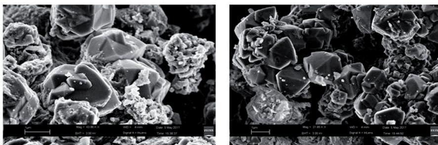
Fig. 5. SEM image of zeolite formed
