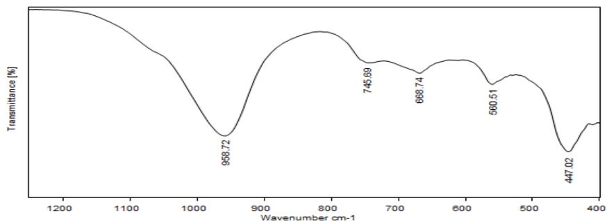
Fig. 4. IR spectra of synthesized zeolite in  $1250\text{--}400\text{ cm}^{-1}$  wave number region
