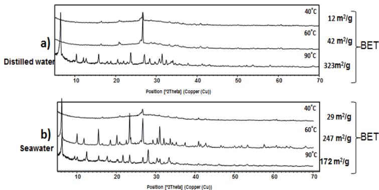
Fig. 3. X- ray diffraction patterns of zeolite crystallization at different temperatures treatment with acid, NaOH/FA 0.75 using : a) distilled water, b) seawater
