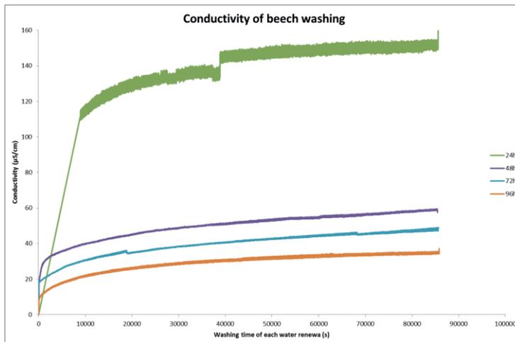
Fig. 2. Conductivity of each washing cycles
