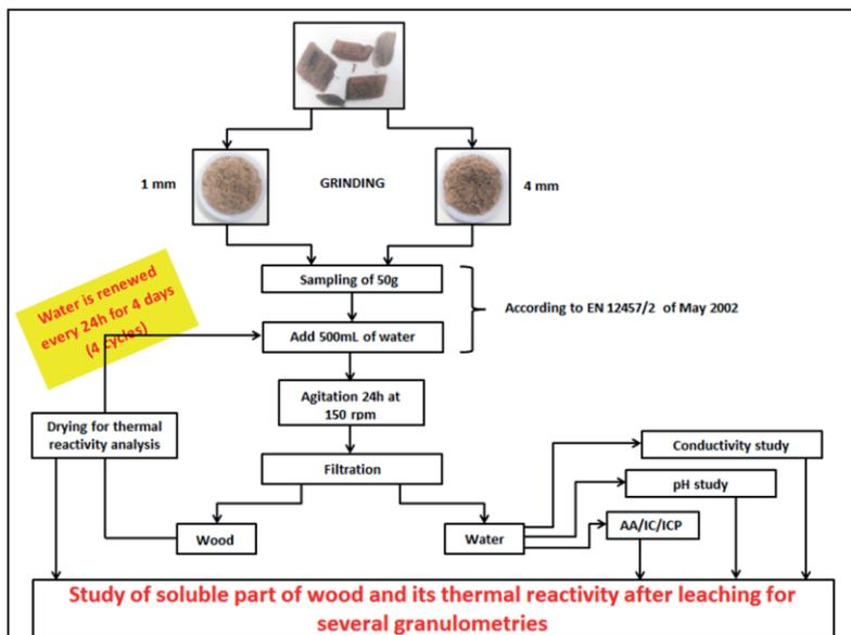
Fig. 1. Experimental washing process
