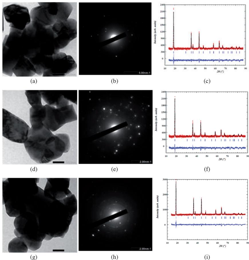
Fig. 4. (a) TEM images (b) SAED pattern (c) XRD pattern of  $\text{Li}_{1.06}\text{Mn}_{1.94}\text{O}_4$  (d) TEM images (e) SAED pattern (f) XRD pattern of  $\text{Li}_{1.08}\text{Mn}_{1.92}\text{O}_4$  (g) TEM images (h) SAED pattern (i) XRD pattern of  $\text{Li}_{1.10}\text{Mn}_{1.90}\text{O}_4$ .
