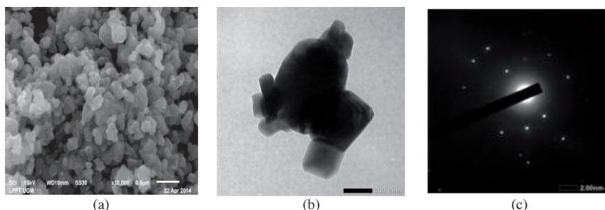
Fig. 1. (a) SEM images (b) TEM images (c) SAED pattern of  $\text{LiMn}_2\text{O}_4$ .
