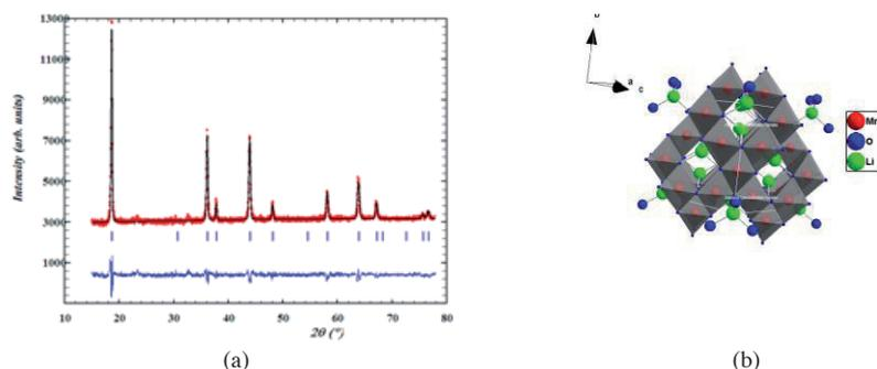
Fig. 2. (a) XRD pattern (b) Microstructure of  $\text{LiMn}_2\text{O}_4$ .
