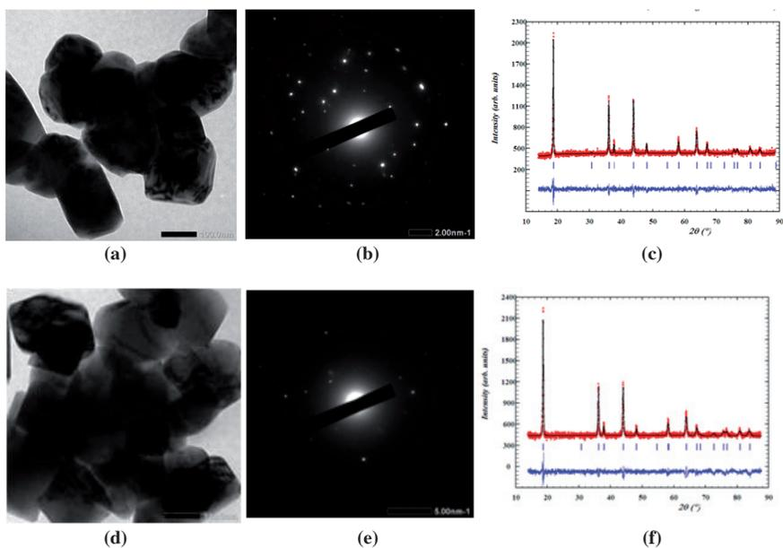
Fig. 3. (a) TEM images (b) SAED pattern (c) XRD pattern of  $\text{Li}_{1.02}\text{Mn}_{1.98}\text{O}_4$  (d) TEM images (e) SAED pattern (f) XRD pattern of  $\text{Li}_{1.04}\text{Mn}_{1.96}\text{O}_4$ .
