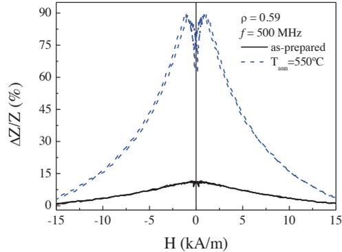
Fig.10. Effect of annealing at 550°C for 1 hour on  $\Delta Z/Z(H)$  dependence of  $\text{Fe}_{70.8}\text{Cu}_1\text{Nb}_{3.1}\text{Si}_{16}\text{B}_{9.1}$  microwire with  $\rho = 0.59$  measured at 500 MHz in comparison with the GMI response of the as-prepared sample.
