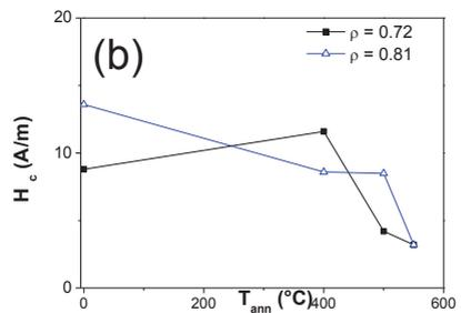
Fig. 9. Hysteresis loops of as-prepared and annealed  $\text{Fe}_{70.8}\text{Cu}_1\text{Nb}_{3.1}\text{Si}_{14.5}\text{B}_{10.6}$  microwires, with  $\rho=0.81$ , at different temperatures measured at fixed magnetic field amplitude of 225 A/m (a) and dependence of the coercivity,  $H_c$ , for the  $\text{Fe}_{70.8}\text{Cu}_1\text{Nb}_{3.1}\text{Si}_{14.5}\text{B}_{10.6}$  glass-coated microwire with selected  $\rho$ -ratio on annealing temperature (b).
