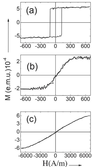
Fig. 1. Typical hysteresis loops of Fe-rich (a), Fe-Co-rich (b) and Co-rich (c) glass coated microwires.
