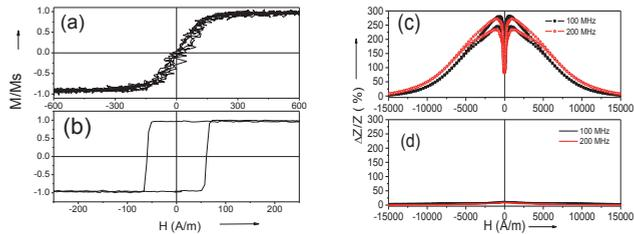
Fig. 3. Hysteresis loops (a,b) and GMI ratio measured in as-prepared  $\text{Co}_{69.2}\text{Fe}_{4.1}\text{B}_{11.8}\text{Si}_{13.8}\text{C}_{1.1}$  and in  $\text{Fe}_{73.8}\text{Cu}_1\text{Nb}_{3.1}\text{B}_{9.1}\text{Si}_{13}$  microwire respectively.
