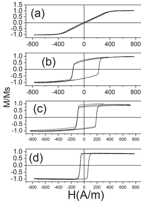
Fig. 6. Hysteresis loops of as-prepared (a) and annealed for 5 min at 200 °C (b), 250 °C (c), and 300 °C (d)  $\text{Fe}_{8,13}\text{Co}_{50,69}\text{Ni}_{17,55}\text{B}_{13,29}\text{Si}_{10,34}$  microwires.
