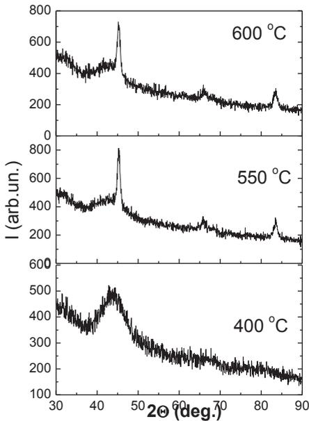
Fig. 8 XRD patterns of annealed microwires:  $\text{Fe}_{70.8}\text{Cu}_1\text{Nb}_{3.1}\text{Si}_{14.5}\text{B}_{10.6}$  with  $\rho = 0.81$ , Annealing temperatures are indicated within each pattern.
