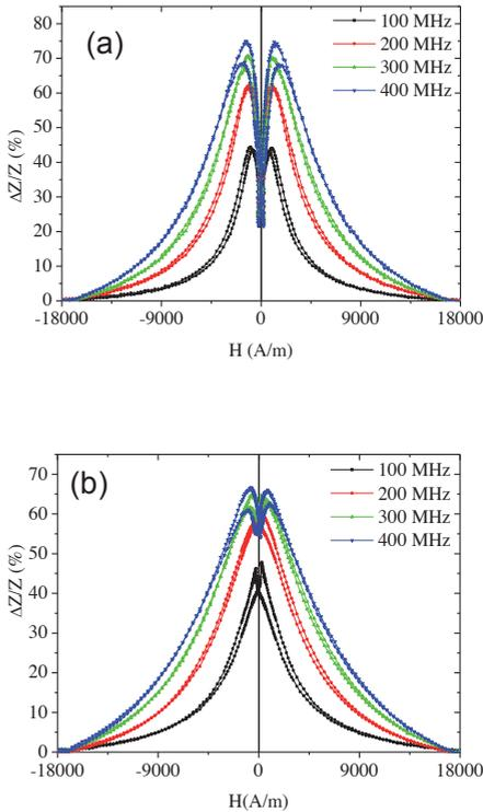
Fig. 7.  $\Delta Z/Z$  (H) dependences of as-prepared (a) and annealed at 200 °C for 5 min (b)  $\text{Fe}_{8.13}\text{Co}_{50.69}\text{Ni}_{17.55}\text{B}_{13.29}\text{Si}_{10.34}$  microwires measured at different frequencies.
