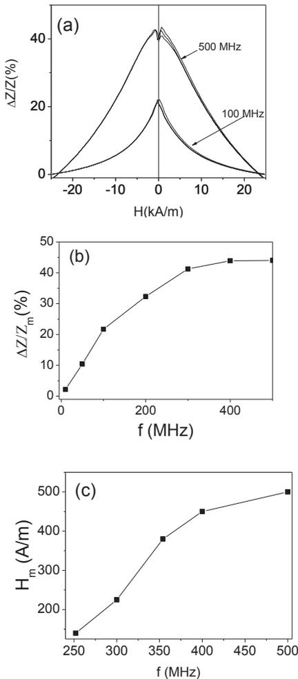
Fig. 4. GMI effect measured in  $\text{Fe}_{75.5}\text{B}_{13}\text{Si}_{11}\text{Mo}_{0.5}$  glass-coated microwire ( $d \approx 18 \mu\text{m}$ ) at different frequencies of AC current (a), dependence of  $\Delta Z/Z_m$  (b) and  $H_m$  (c) on  $f$ .
