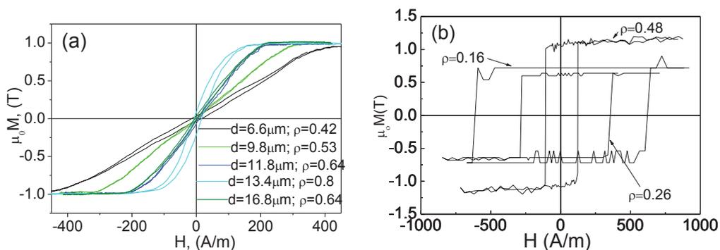
Fig. 2. Hysteresis loops of  $\text{Co}_{67.1}\text{Fe}_{3.8}\text{Ni}_{1.4}\text{Si}_{14.5}\text{B}_{11.5}\text{Mo}_{1.7}$  microwires with different geometry (a) and of  $\text{Fe}_{70}\text{B}_{15}\text{Si}_{10}\text{C}_5$  amorphous microwires with with  $\rho = 0.63$ ;  $d = 15 \mu\text{m}$  (a);  $\rho = 0.48$ ;  $d = 10,8 \mu\text{m}$  (b);  $\rho = 0.26$ ;  $d = 6 \mu\text{m}$  (c);  $\rho = 0.16$ ;  $d = 3 \mu\text{m}$  (d).
