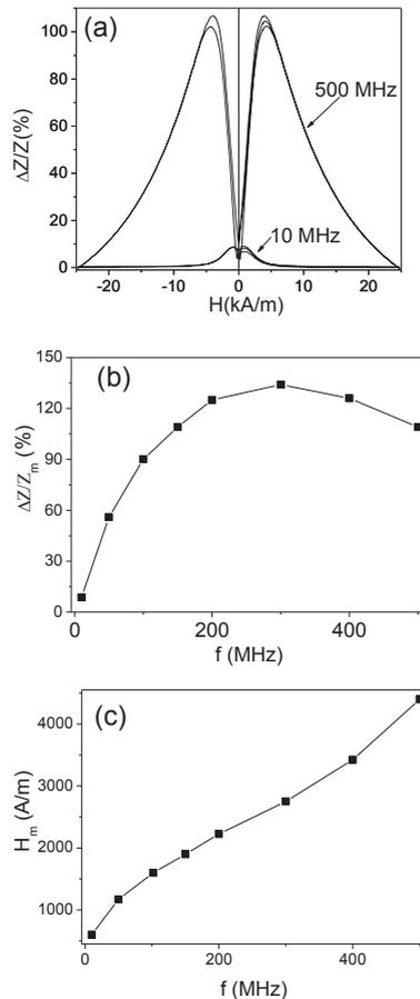
Fig. 5. GMI effect measured in  $\text{Fe}_{3.7}\text{Co}_{69.8}\text{Ni}_1\text{Si}_{11}\text{B}_{13}\text{Mo}_{1.5}$  glass-coated microwire ( $d \approx 19 \mu\text{m}$ ) at different frequencies of AC current (a), dependence of  $\Delta Z/Z_m$  (b) and  $H_m$  (c) on  $f$ .
