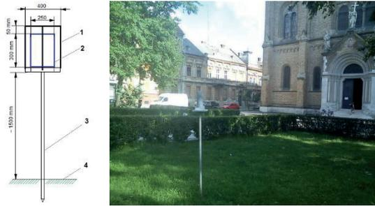
Fig. 1. TSP collection setup. 1 – bird protection; 2 – collecting vessel; 3 – stack; 4 – ground; and view of the collecting site location.
