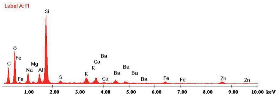
Fig. 5. Sample analysis with EDS.
