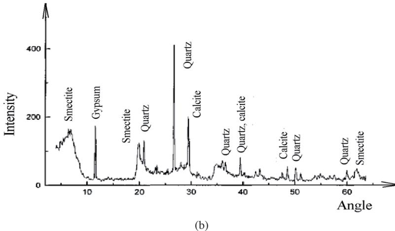
Fig. 1. Diffractograms of Urangaiskaya (a) and Akzharskaya (b) bentonite clays.
