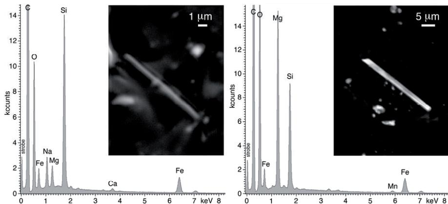
Fig. 2. Energy dispersive spectra and the relative back scattered electron. SEM image of an amosite (left) and a chrysotile (right) fibre.
