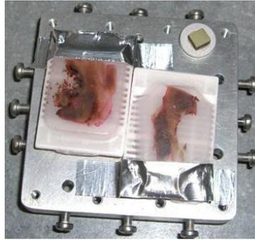
Fig. 1. SEM specimen holder with two paraffin embedded specimen.
