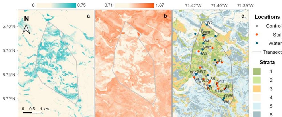
Fig. 2. Two covariates used in the SRSD and locations. a) NDVI, b) iron oxide ratio, c) k-means strata and studied locations. The labelled points correspond to sites sampled for glyphosate analysis. Sentinel-2 images were acquired from Copernicus Open Access Hub and pre-processed using SNAP V. 7.0.0. Plotted with QGIS V. 3.12
