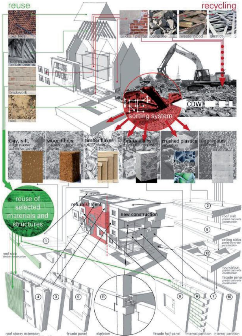
Fig. 2. Conceptual architecture of RE<sup>4</sup> Project
