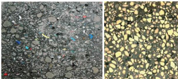
Fig. 1. Cross section of SUS-CON concrete samples made of recycled binders and plastic aggregates
